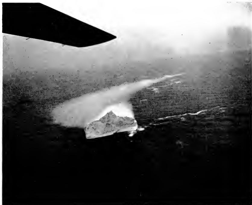
FIGURE 17.—Results of bomb drop on 1 June 1959. The incendiary bomb cluster produced much smoke and steam but appeared to have little effect on the disintegration of the berg. The Ice Patrol Vessel, USCGC ANDROSCOGGIN, is standing by to evaluate results.
